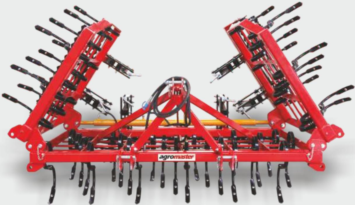
4 Row S-Tine Foldable Tiller is a secondary soil tillage machine is mounted to tractor's hydraulic lifting unit and universal three point linkage system, hydraulically mounted type machine. Therefore transportation to the field can be easily done.
