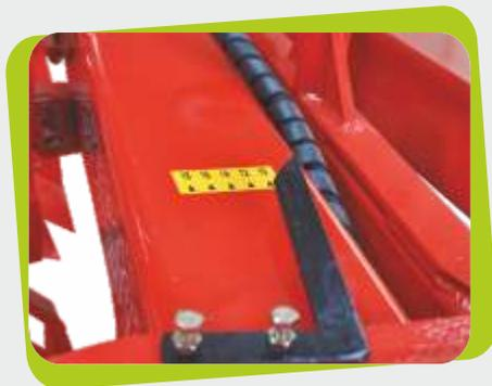
The width between bodies can be easily adjusted through 1nc adjustment of hydraulic control mechanism.
