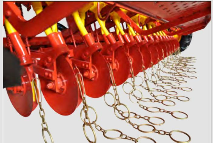
Chains for field levelling for getting layer of mulched soil
