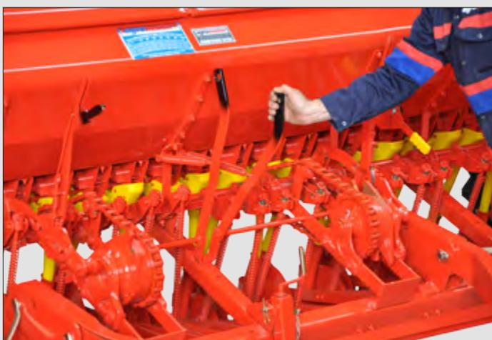
Mechanical lever for adjustment of sowing position of disc
