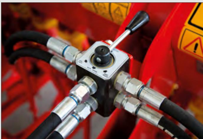
Valve to change sowing position of right, left and both side discs
