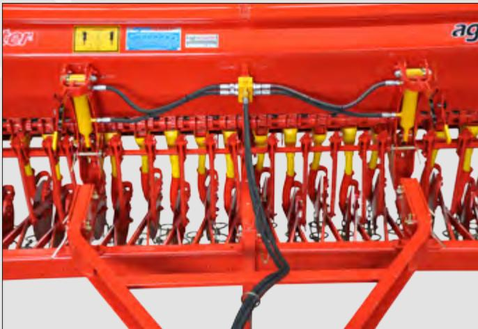
Hydraulic mechanism for adjustment of sowing position of discs
