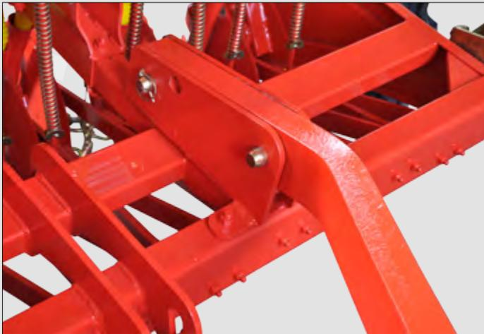
Lifted draw bar fixing mechanism
