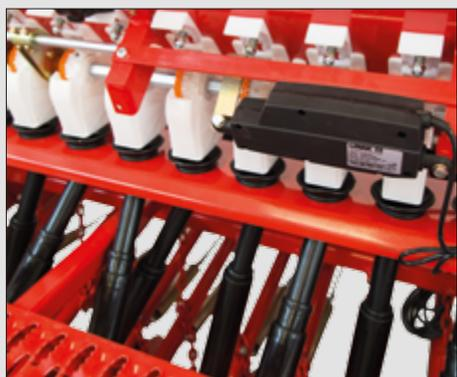
Electric or solenoid (optional) valves for tramline control
