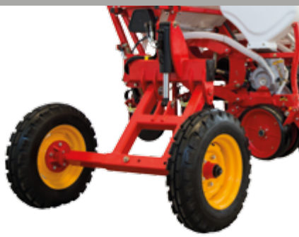
Side drawbar in transport position
