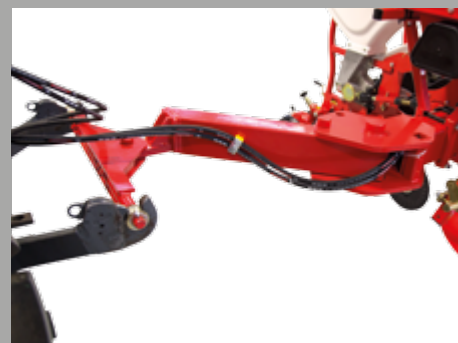
Side drawbar in transport position
