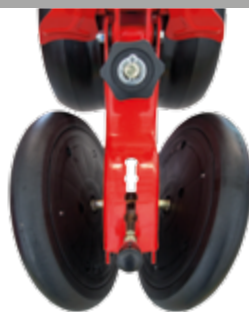
V shaped rear roller for pressing down and closing seed beds
