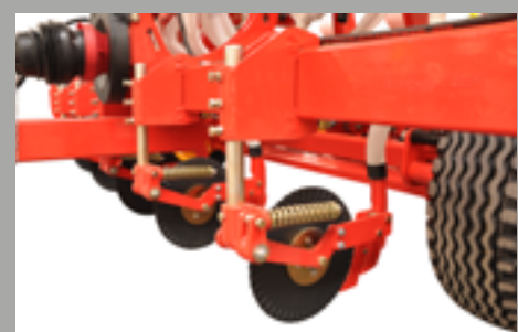
High pressure turbo fertilizer disc coulters
