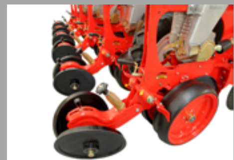
V shaped cast iron press wheel
