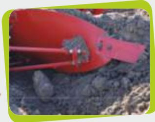
Moldboard extension part provides to overturn cut soil layer better.
