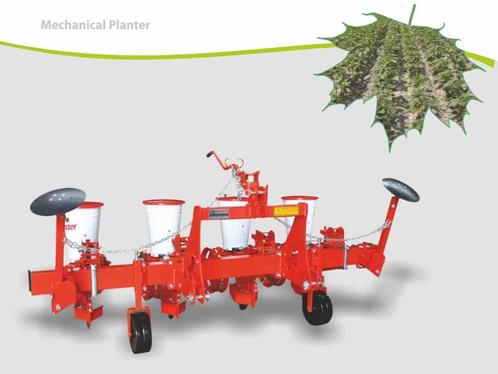
Mechanical planter can be used for precise seeding. Different type of seeds like corn, sun flower, cotton, sugar beet, soybean, peanut, and chickpea can be sowed on single row with this machine on every kind of cultivated soil.
