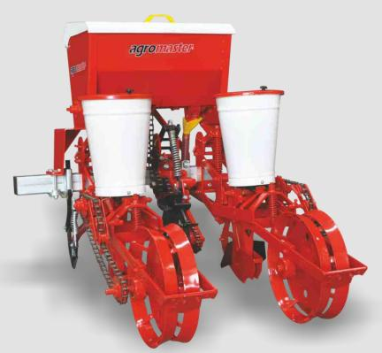
Mechanical planter has 2, 4, 5 and 6, seed unit, sowing foot, disc coulter and disc. It is produced with fertilizer hopper and without fertilizer hopper. Seed machine is operated by means of mechanical system. Mechanical planter is operated with hydraulic lifting lever and universal three point linkage system. Machine can be transported easily to the field.
