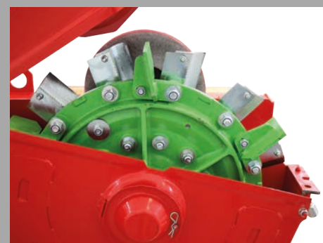
Powerfull impeller with 12 knives and 6 launchers
