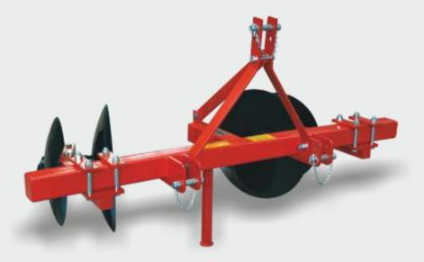
dimensions are 660x6 mm and 560x4,5 mm. The hardness value for discs is 50-55 rh and they are durable to wear and breakage.
