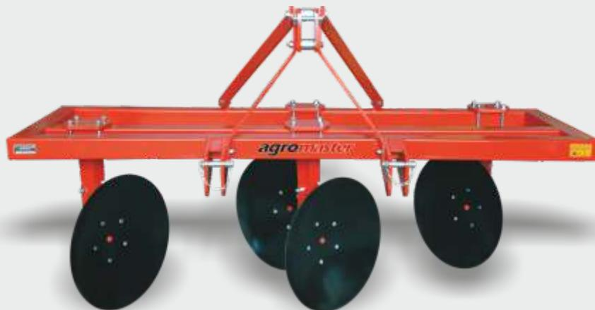
These Ridgers are mounted to tractor's hydraulic arms and linkage system. So it is very easy to transport these ridgers to field. These machines are used for making one and two rows ridgers and opening canal. According to user's wishes discs angels can be arranged (0-23°) to make canal or ridge. Also disc connection legs of machine can be arranged 20°-50°. By means of the adjustable legs of machine row spaces of canals and ridges can be adjusted 45-100 cm.
